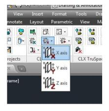
Users May Select to Slice a Cloud on the X, Y, or Z Axis of the Model Space
